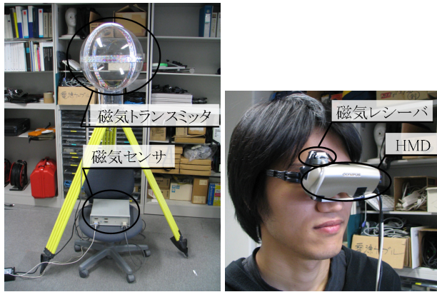
図 14 磁気センサ(左)と磁気レシーバ付き HMD(右) Magnetic sensor (left) and receiver attached HMD (right).
