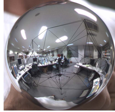
Figure 7. Mirror region is triangulated based on tracked feature points with Delaunay triangulation method.
