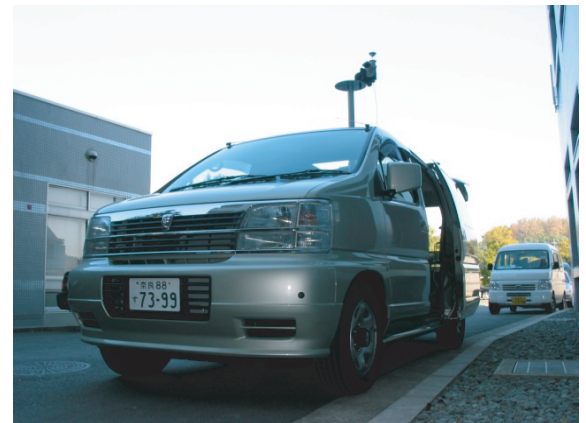
Figure 3. Omni-directional camera acquiring the scenery surrounding the automobile
