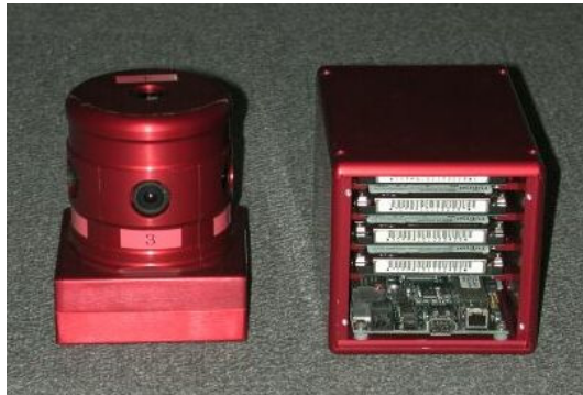
Fig. 2. Omni-directional multi-camera system; Ladybug.
