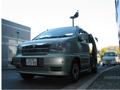
Fig. 6. Appearance of car for omni-directional video acquisition.
