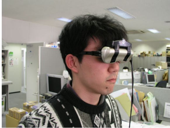
Fig. 4. HMD (Head Mounted Display) with gyro sensor.
