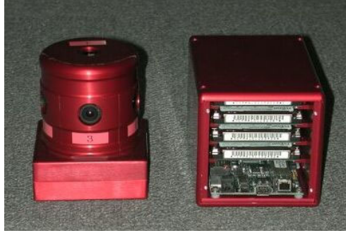
Figure 1. Camera head (left) and storage unit (right) of Ladybug.
