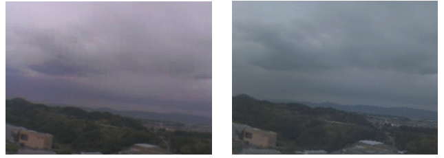
(a) Without ND filter (image captured from bottom of airship). Average intensity: (R, G, B) = (111.5, 108.3, 119.7) . (b) With ND filter (image captured from top of airship). Average intensity: (R, G, B) = (95.1, 103.5, 111.9) .
