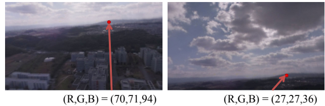
Fig. 22 Examples of view direction dependent tone-mapping: The intensity of the same position in the scene varies according to the view direction.
