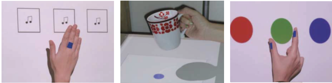
Figure 4: The post-stroke rehabilitation system proposed by Hondori et al [4]. Users are directed by the system to perform specific hand motions. In the first column, users reach for boxes to play sounds; in the second column, users pour virtual water on the blue spot; in the third column, users grasp randomly positioned circles.
