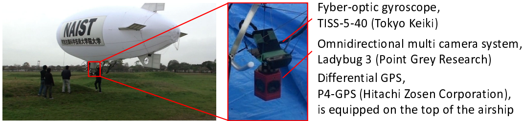
Figure 3.1. Unmanned airship and mounted sensors
