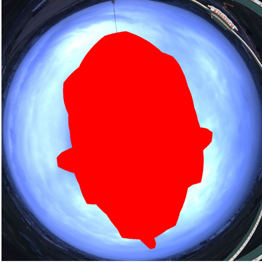
(a) A sky image in equisolid angle projection, where the missing area is masked.
