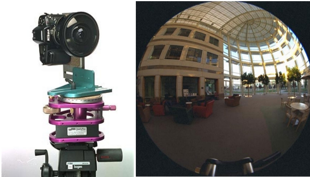
Figure 2.1. Fisheye camera and acquired image in [XT97].
