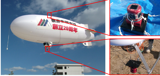
Figure 3. Unmanned airship and omnidirectional cameras. Two cameras are mounted on the top and bottom of the airship. ND filters are attached to the camera on the top. A GPS antenna is also mounted atop the airship.
