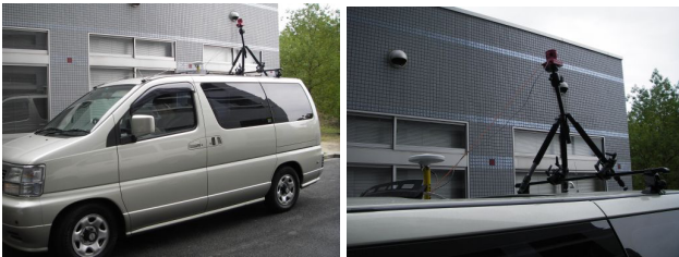
(a) Data acquisition vehicle. (b) GPS receiver (left) and OMS (right).
